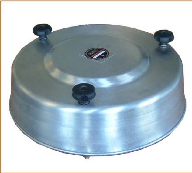
The PRV is the last line of defence and should never have to be used. The Hycontrol system allows for optional full testing of this vital component. Using small air cylinders, the system can lift the valve to check operation, with proximity switches detecting correct lifting and closing.
