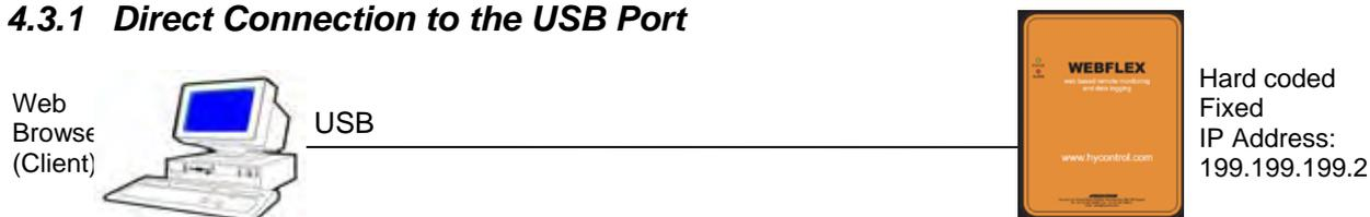
A direct USB connection to the WebFlex can be made in two ways. A temporary connection or a permanent connection can be made between a PC and the USB connector inside the unit. The cable length is limited to 5 meters (15 feet).
