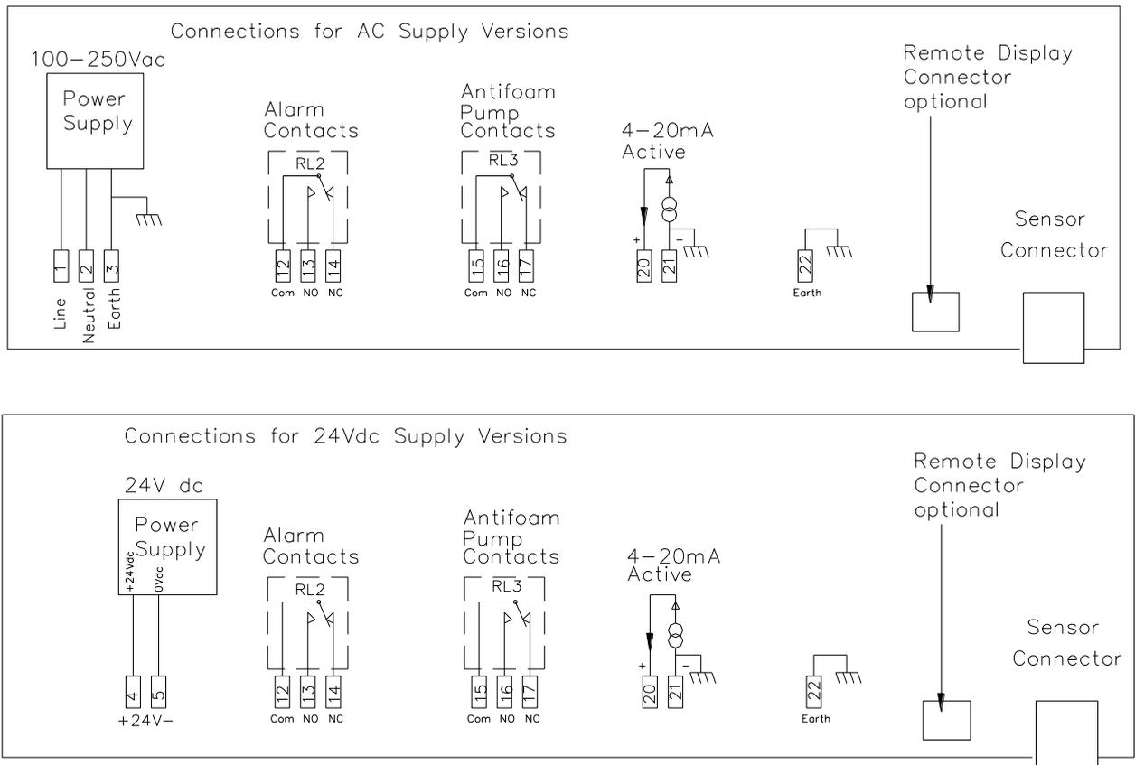
The system will require minimal setting-up and commissioning before use. In most cases the factory set up will be adequate for the initial operation. When the system is powered up initially it should start to sense foam immediately if any is present and transmit a signal via the 4-20 ma output. The 4-20ma range is set to cover 100% of the sensor length. The display reads the foam level in mm from the end of the sensor and % coverage of the sensor.
