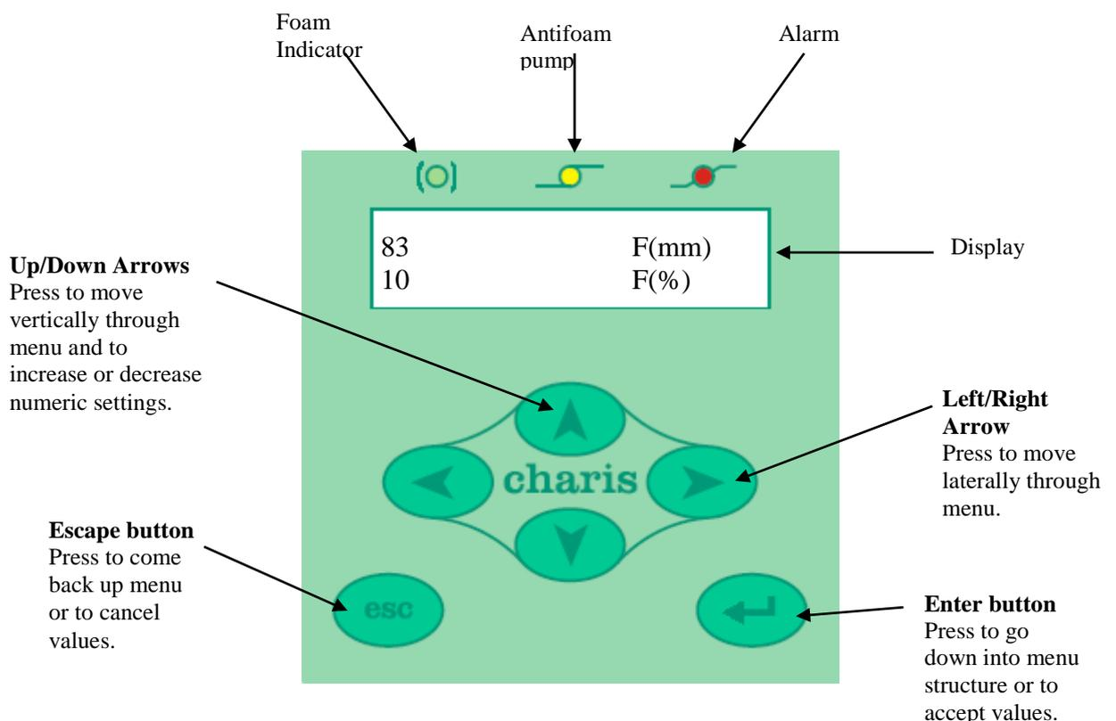
After power up the display will show the control screen. The control screen is the main operating screen and shows two continually updating readings. The user can set which two readings are displayed.
