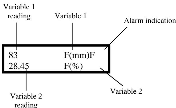
The variables displayed are selected in the Display Menu (see section 4.4) with variable 1 on the first line of the display and variable 2 on the second line. The resolution of the variable readings (the number of decimal places that are displayed for a numerical measurement) can be changed in the Display Menu with Display Resolution 1 referring to variable 1 and Display Resolution 2 referring to variable 2.
