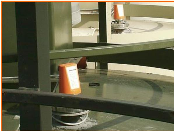
Hycontrol's Reflex VF Series range of TDR products is ideal for this application and can be used for the measurement of liquids, powders and granules. The technology, originally used to detect breaks in subsea cables, uses pulses of low power microwaves sent along the conducting probes. At the point where the waves meet the air-product interface, they are reflected by the product back along the probe.
