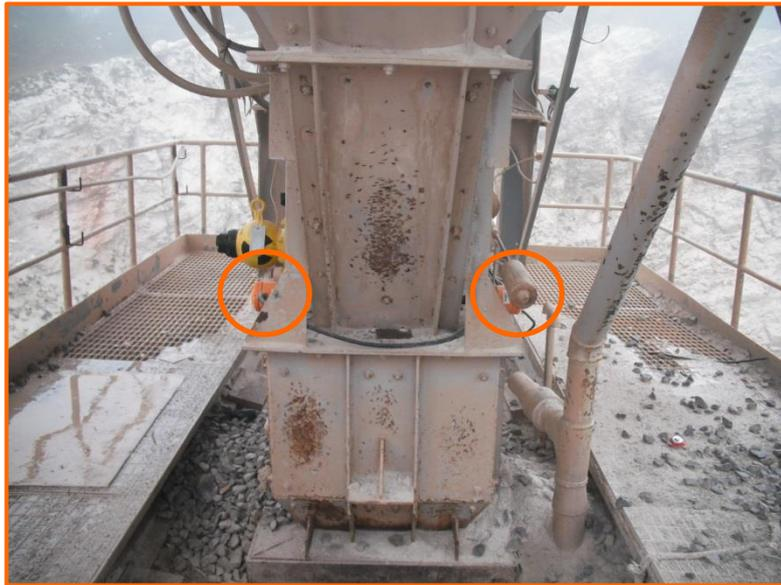
dielectric materials such as refractory bricks, ceramics, plastics and polymers. This means that low cost replaceable windows can easily be fitted into the sides of a chute, vessel or container, keeping the process closed with no disruption to material flow and the microwave transmitters/receivers at arm's length away from the harsh environment. The system is extremely easy to set up and calibrate and the microwave
