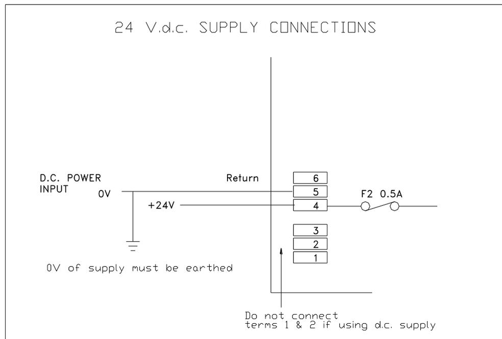
The return terminal can be used to connect to the vessel if it is not earthed, to provide a return signal. In most installations it is not required. See section 3.4 for details.
