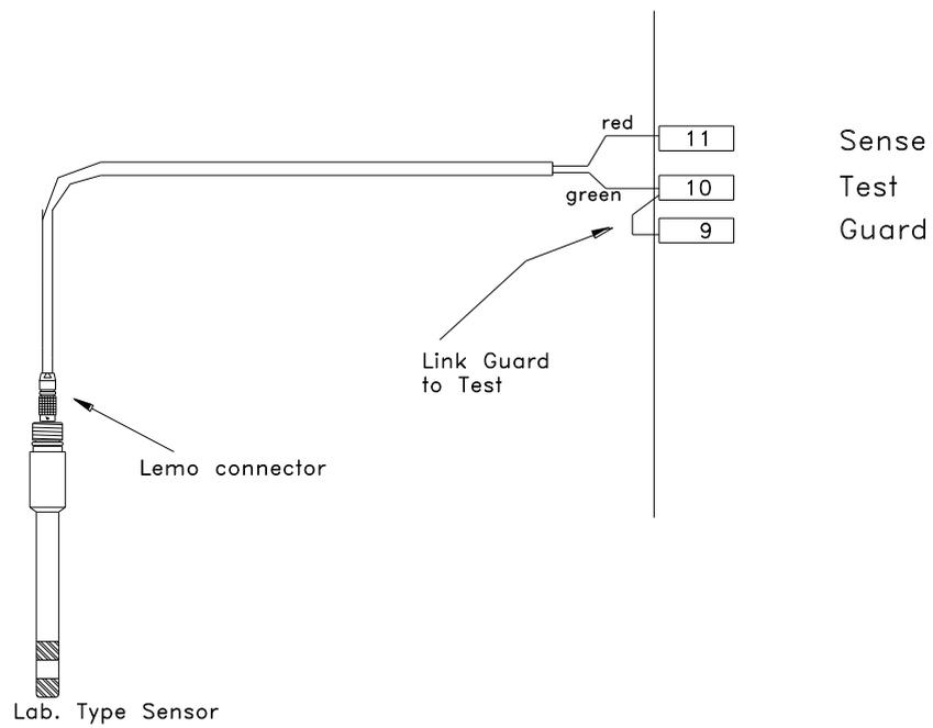
Use unscreened twisted pair cable, length must not exceed 20m
