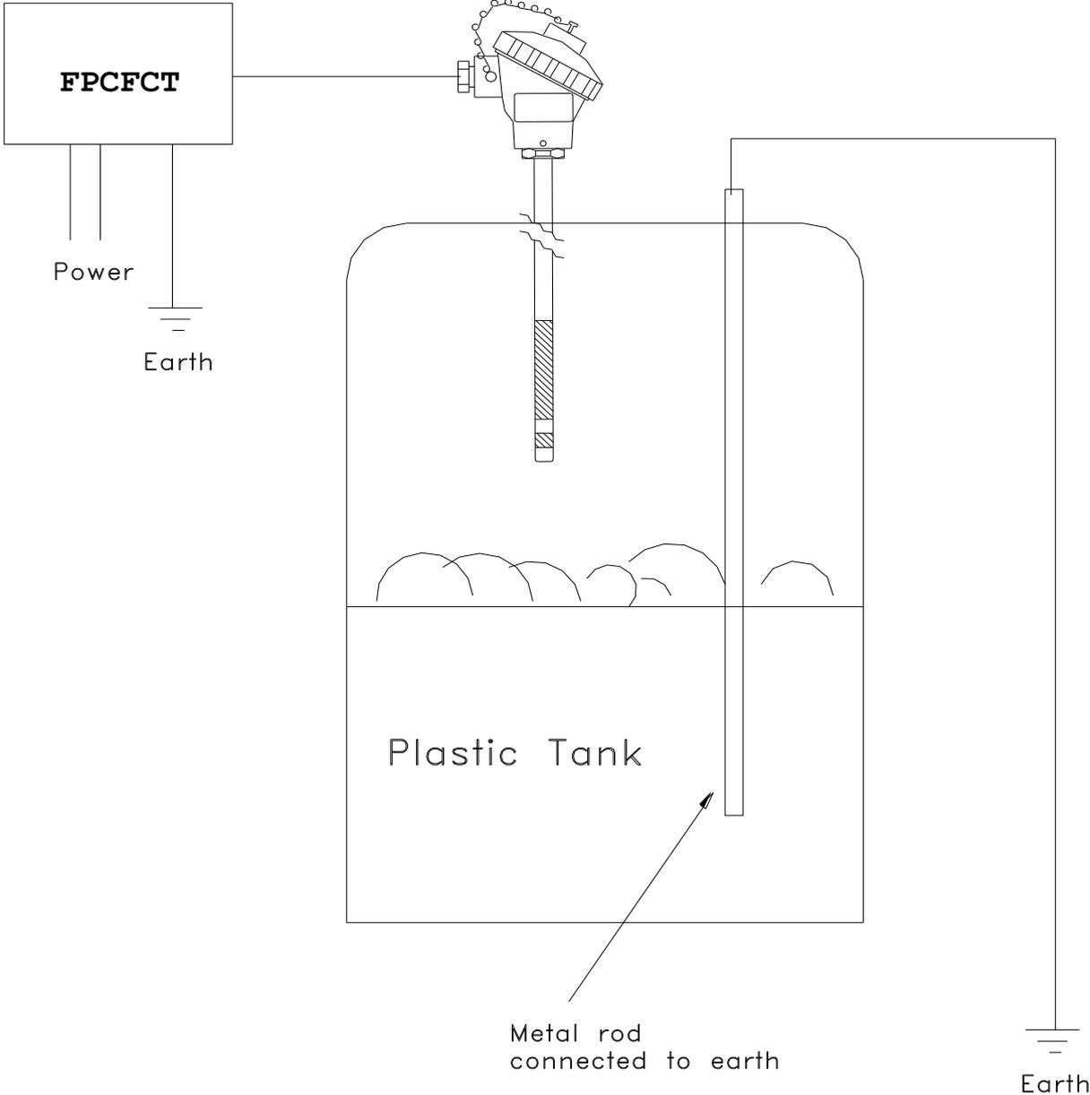
When using a plastic tank it is necessary to use a metal electrode or pipe connected to earth (ground) to supply a signal return path.
