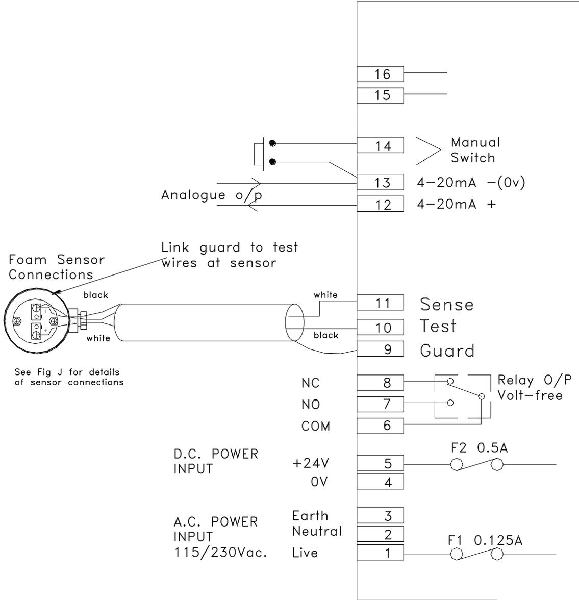
use SCREENED twisted pair cable for sensor
