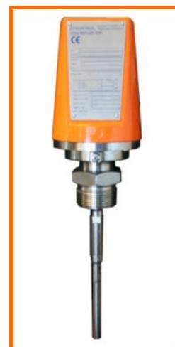
the bitumen levels are measured using Hycontrol's high-temperature VF03 TDR sensors. The stainless steel probes are usually fitted to flanges at the top of the tanks and extend down into the hot bitumen. The probes allow a very narrow measuring profile up to a maximum range of 24 metres and this is particularly useful for measurements in tanks which have internal structural supports.
