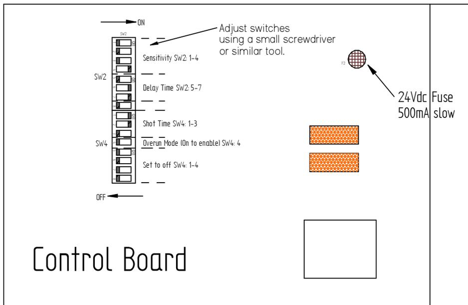
Switch settings are used to adjust the sensitivity and the Delay and Shot times. The switches are only read at power-up. To make adjustments switch off the power to the controller then make the adjustments and then switch power on again.
