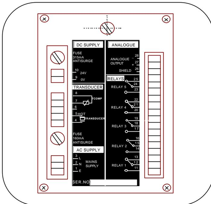
**b. Electrical and Transducer Connections**
