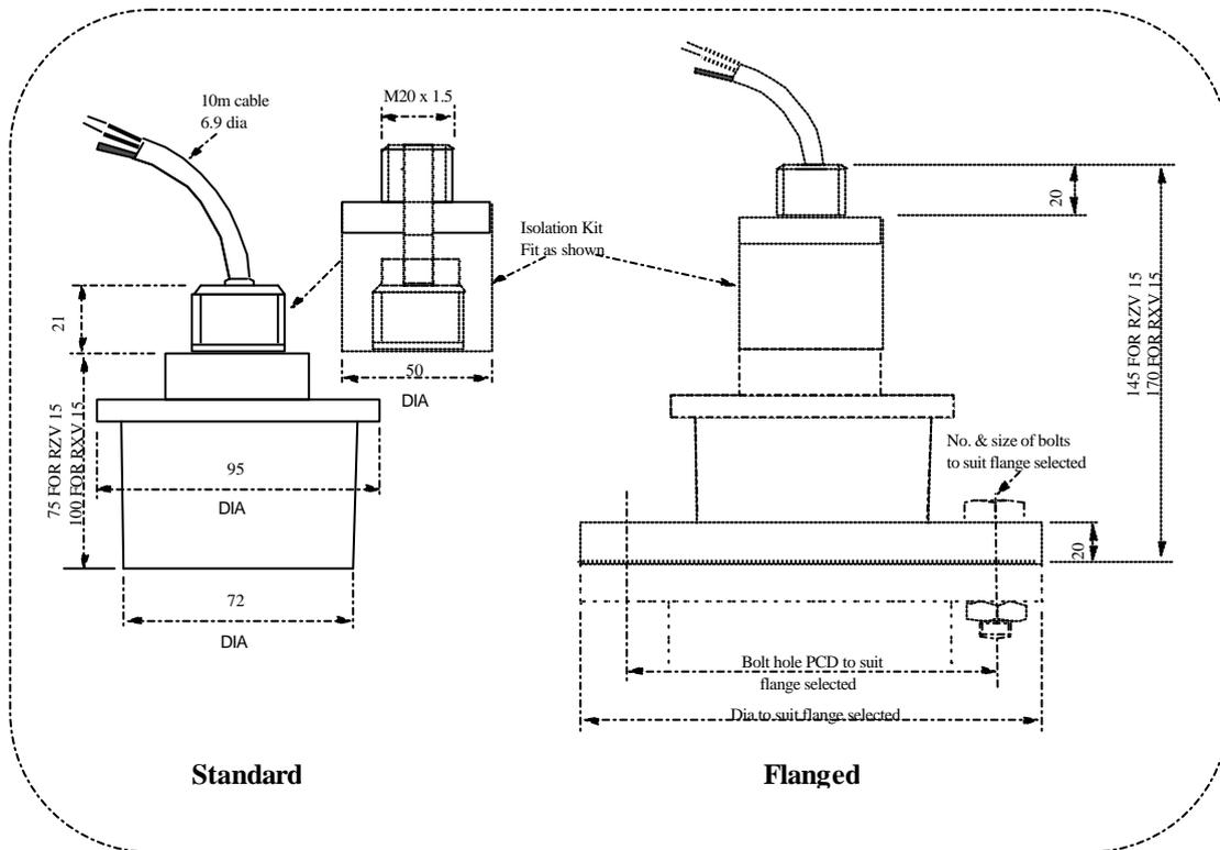
An isolation kit is provided with each transducer to minimise any ringing transmitted through the mounting structure.
