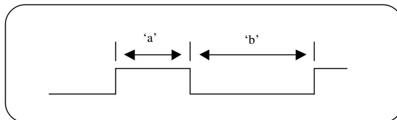
The time 'a' is set by Pr.12 and 'b' is set by Pr.13 in seconds, this allows any shape drive train to be defined.
