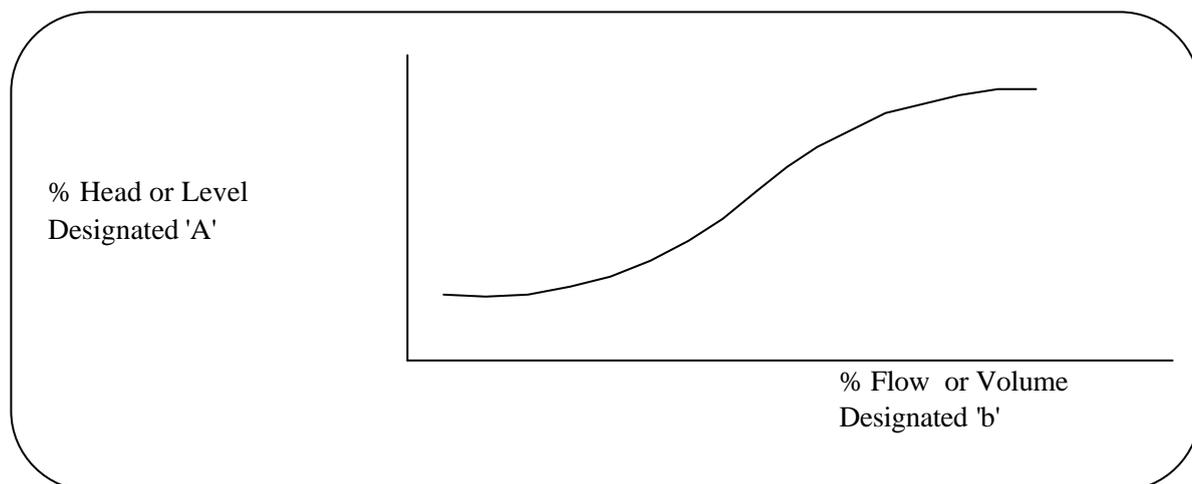
The profile data is input into Pr.44 which, when accessed, [Pr.44, 'DSP', 'ENT'] will display 'A1', which means the data pointer is at value 1 on 'A' data. The values can be displayed and changed as required.
