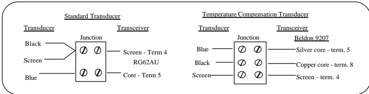
**Figure 7: Transducer Wiring for Differential Mode**
